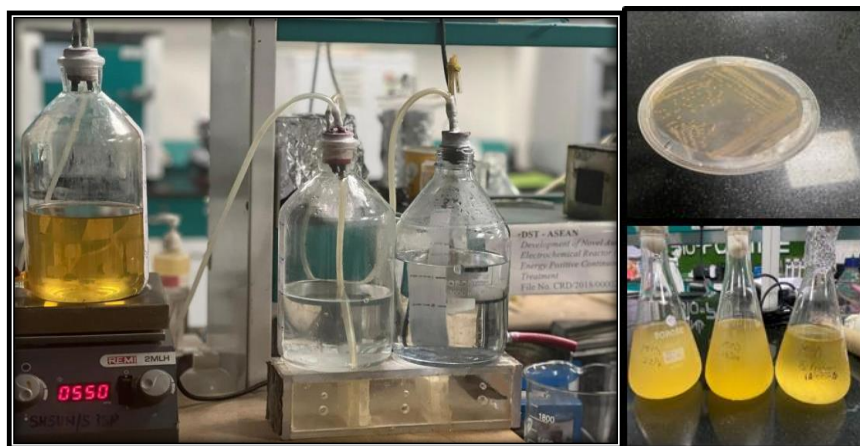
Figure 2: Biohydrogen production set-up using water displacement procedure and Inoculum Enrichment
